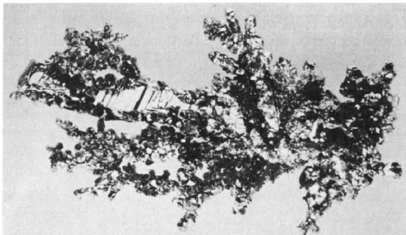
Fig. 1. Refined titanium dendrite. Courtesy of J. C. Priscu, Titanium Metal Corporation of America, Henderson, Nevada.
